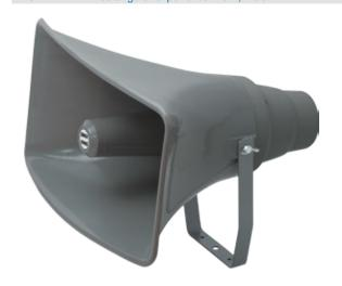
TR1-B, TR2-B and TR3-B exponential horns are made of grey Moplen. They are unbreakable and weather-proof. Each horn has a swivelling bracket for securing it in place and a rear cap able to contain a UT35 or UT60 impedance-type magneto-dynamic unit or a UT60-T unit with a 100V transformer, not included in the supply (refer to the appropriate technical table).
