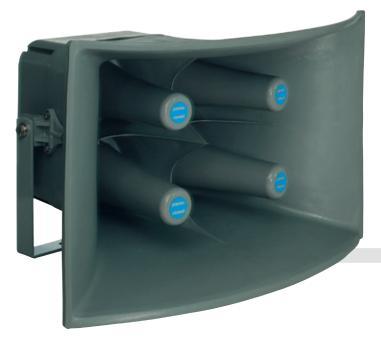
The **TR400-SX** horn can fit four **UT60** (60 W/16  $\Omega$ ) or **UT150** (150 W/16  $\Omega$ ) compression units, supplied separately. The sound waves generated by the single units are synchronised when their acoustic pressure is still in the initial expansion phase. Reinforced fibreglass material. Very high efficiency combined with perfect intelligibility of speech. These features
