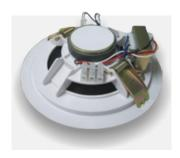
The speaker units for ceiling-mounting of the **C51** range consist of an ABS structure with a RAL 9016 white-painted grille. They feature a compact size and an excellent acoustic performance. Each unit has handy tough spring-type hooks that make it easy to fasten securely to a false ceiling. A transformer for connection to a 100V constant-voltage line is included in the supply, with selectable power-output steps.
