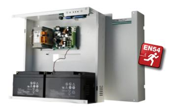
The **W-MS24/WF** power supply and battery-charging unit consists of a switching type PSU with protection against short circuits and overloading and a card for managing controlled dynamic recharging of sealed lead batteries (tested regularly) and alarm outputs, a self-testing function and LEDs for signalling 16 different system statuses.
