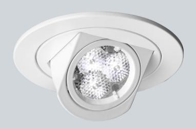
The DL9 down light has full directional adjustability to suit a wide range of applications. The bezel allows both rotation and angling of the LED with the central scoop adjusting to almost vertical.
