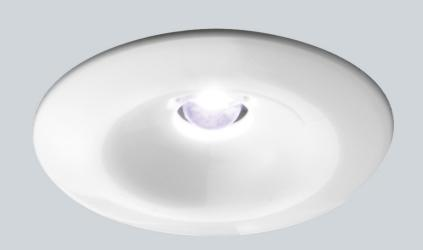
With a depth of just 10mm, the DL3 is ideal for very shallow recessing depth requirements. With a simple push fit arrangement, these fittings are secured with a friction fit into the aperture. The petit dimensions, DL3 is just 24mm diameter, make this an ideal solution for adding visual interest to a wall or ceiling or for discreet feature display lighting, within a display case for example.
