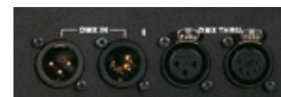
DMX input/output interface (XLR 3-5 male/female)
