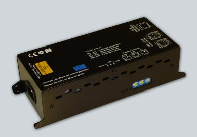
The patented iDrive UL is one of the first high powered LED drivers which can drive 3 channels of LEDs at 350mA and up to 48V DC that is approved to UL and cUL specifications. In additional, the iDrive UL is approved to CE 61347-2-13 which all LED drivers must meet come July 1st 2009. It has also been designed to make installation simple and to save time by using standard power and DMX connectors with a unique user interface to control all iDrive UL functions.
